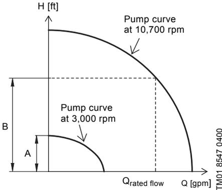
**Fig. 6** Pump curves at 3,000 rpm and 10,700 rpm
