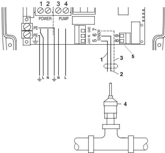
Fig. 20 Electrical connection of the CU 301
