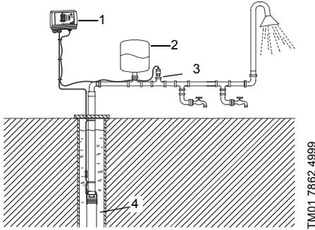
**Fig. 1** Example of a system with constant-pressure control
