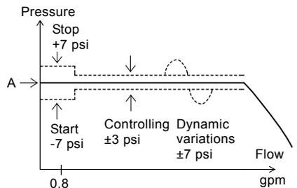
**Fig. 5** Possible pressure variations during constant-pressure operation
