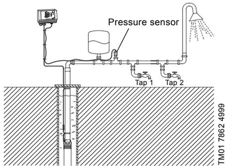
Fig. 7 Pressure sensor position
