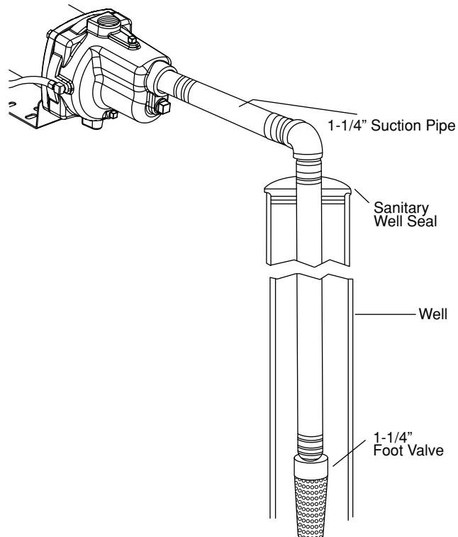
for a cased/dug well. Either can be used for pumping from a lake or stream, provided the end of the suction pipe is also protected by a strainer. Special care should be taken to ensure that all suction fittings are tight and sealed. Otherwise, the pump cannot be primed or will lose prime over a period of time.
