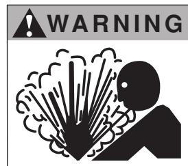
**WARNING HAZARDOUS PRESSURE:** Do not run pump against closed discharge. Release all system pressure before working on any component.
