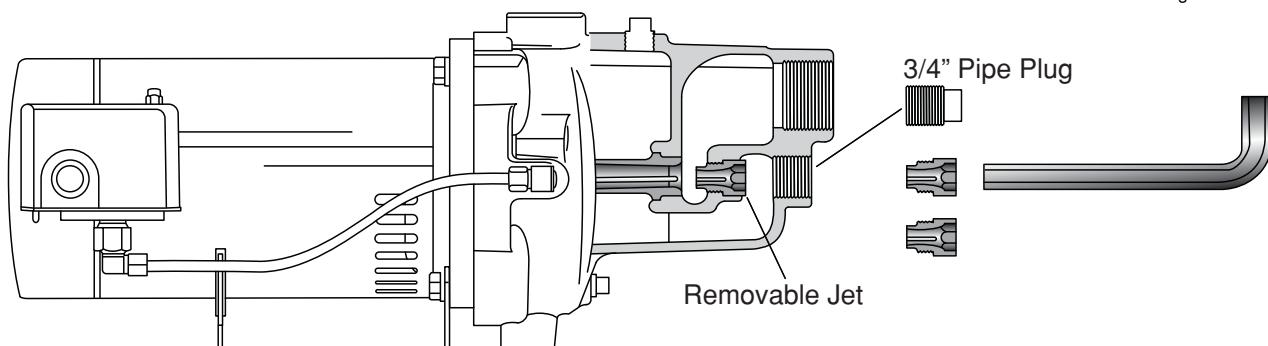
If your pump must be drained for service or to prevent damage from freezing, remove the drain plug from the pump case.
