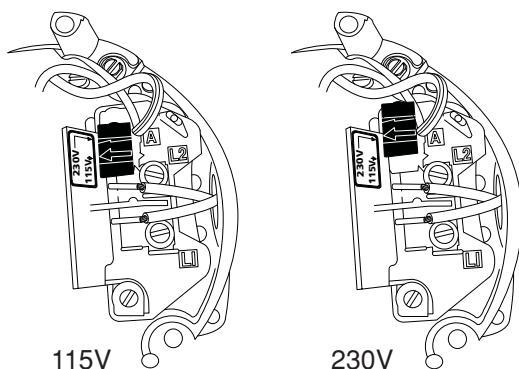
**NOTICE:** Check motor terminal cover or nameplate for wiring instructions. The essential pump motor facts are as follows:
