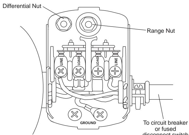
The pressure switch is set to start the pump at 30 psi and to stop at 50 psi. **THE PRESSURE SWITCH SHOULD NOT REQUIRE ADJUSTMENT FOR A TYPICAL PUMP INSTALLATION.** Adjust the switch only if necessary using the following procedure:
